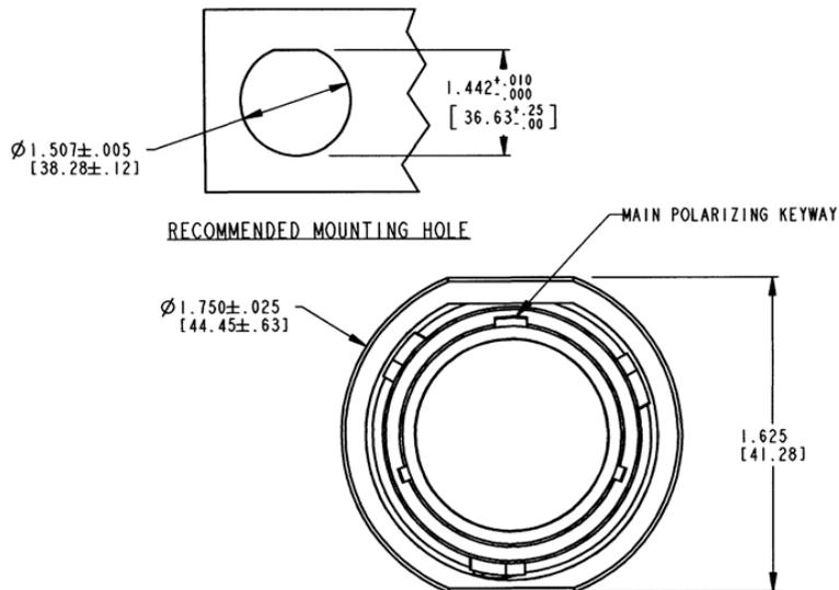
To mount the circular multiway connector in the battery box, a hole of the following dimensions needs to be cut in the battery box.
