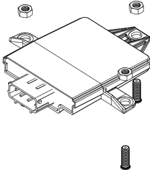
Install the ECU using three M8 hex socket head screws (not included) with a minimum engagement length of 7.2mm. It is recommended to use spring washers or lock washers to secure the screws. The ECU is IP67 rated and can be installed outside the battery box, however should not be mounted in any area susceptible to road dirt/stones being thrown up at it.
