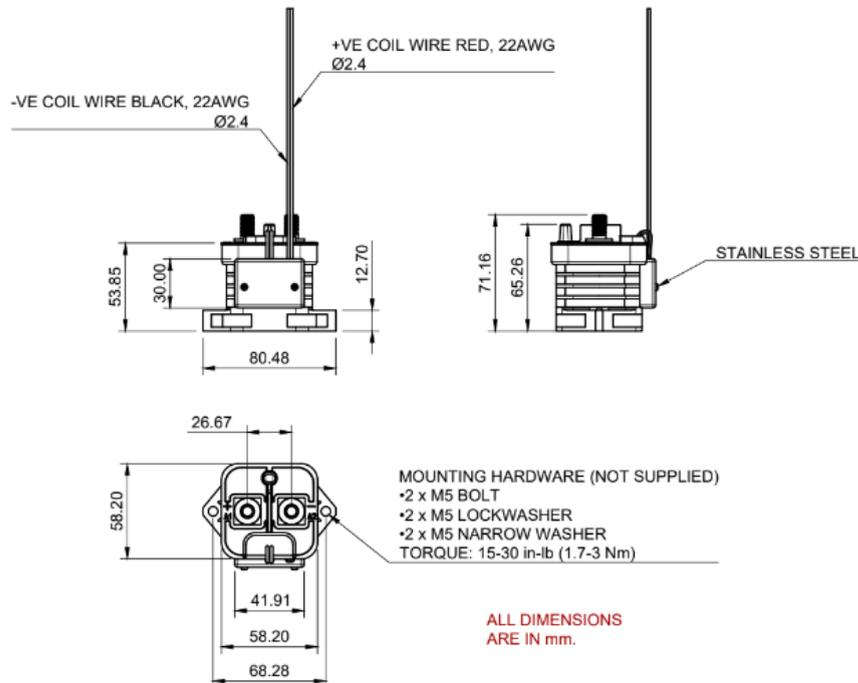
For the CCS contactors please refer to the diagram for mechanical properties. Spring washers are required on the power terminals and the retaining nuts should be tightened to 8.8-11Nm. It is recommended to make sure the busbar and contactor terminals are clean of all contaminants to ensure good contact.
