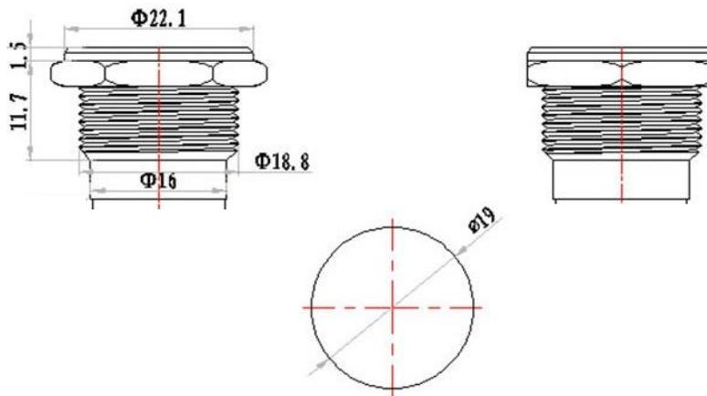
Mounting hole diameter 19mm
