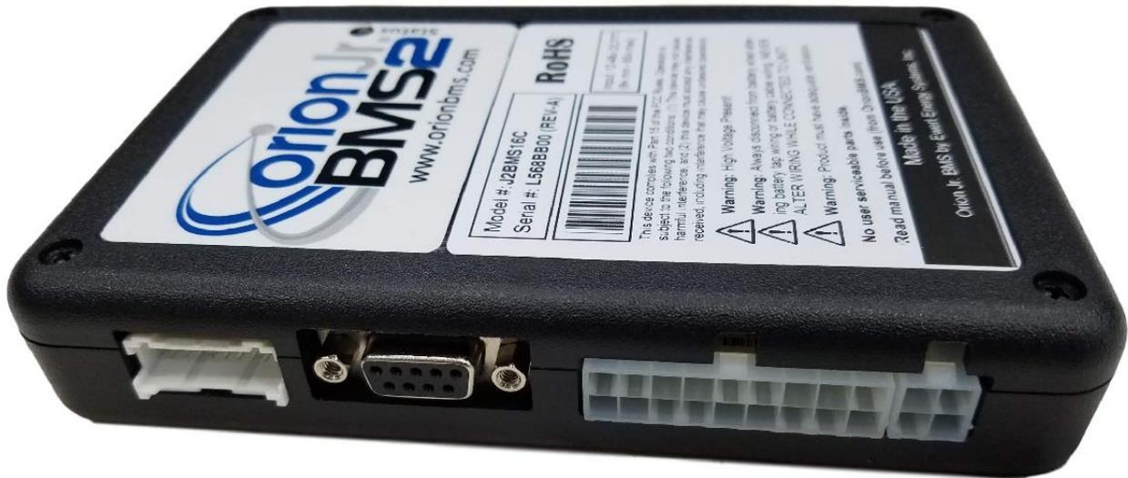
The Orion Jr. 2 BMS by Ewert Energy Systems is designed to manage and protect Lithium ion battery packs and is suitable for use in stationary energy storage and small mobile applications such as golf carts and material handling equipment.
