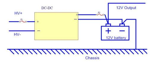
Both the HV and LV side needs a fuse. For the HV side a fuse size of 40-50Amp is recommended.
