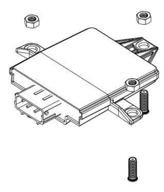
Install the ECU using three M8 hex socket head screws (not included) with a minimum engagement length of 7.2mm. It is recommended to use spring washers or lock washers to secure the screws. The ECU is IP67 rated and can be installed outside the battery box, however should not be mounted in any area susceptible to road dirt/stones being thrown up at it.
