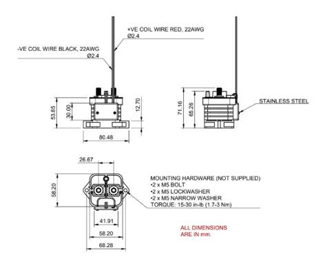
For the CCS contactors please refer to the diagram for mechanical properties. Spring washers are required on the power terminals and the retaining nuts should be tightened to 8.8-11Nm. It is recommended to make sure the busbar and contactor terminals are clean of all contaminants to ensure good contact.
