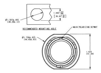
To mount the circular multiway connector in the battery box, a hole of the following dimensions needs to be cut in the battery box.
